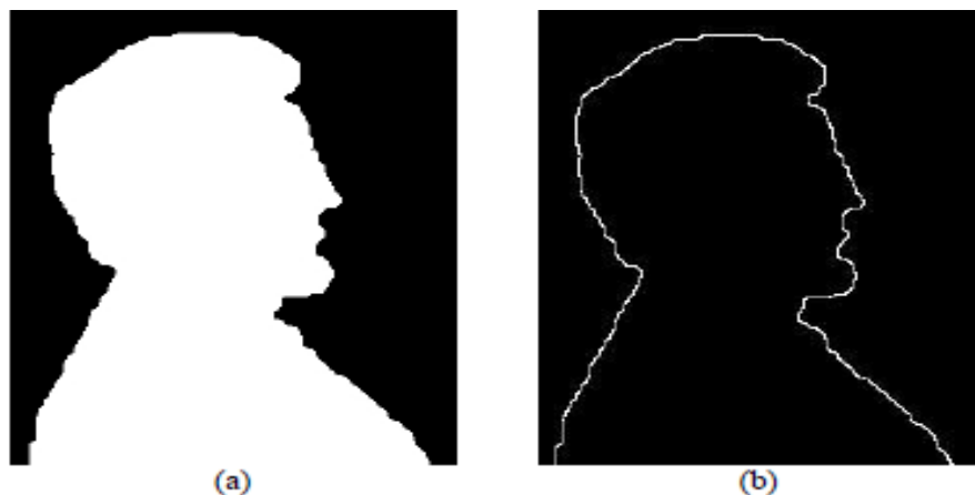
Figure 12.2 (a) Binary image. (b) Object boundary extracted using the previous equation and 3 \times 3 square structuring element.
