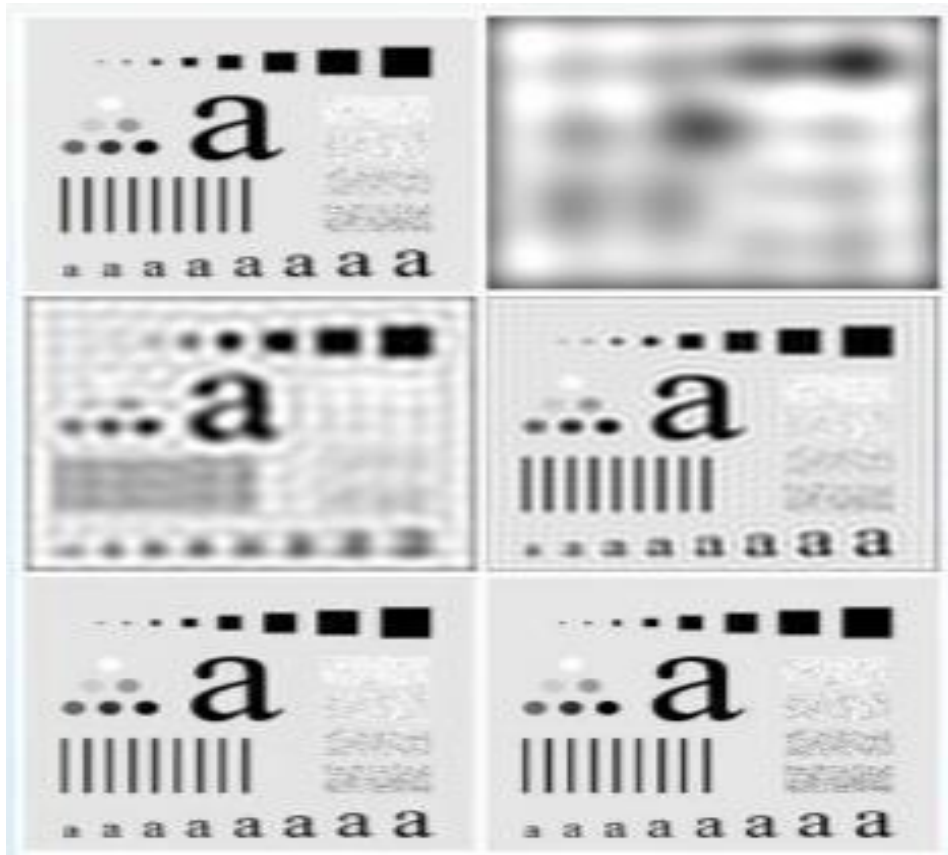
Fig: (a) original image, (b)-(f) Results of filtering using ILPFs with cutoff frequencies set
