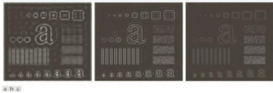
Fig.. Results of high-pass filtering the image in Fig.(a) using an IHPF with D_0 = 30, 60 , and 160.
